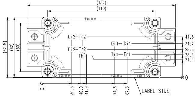
Tr1/Tr2: IGBT, Di1/Di2: FWD, Th: NTC thermistor
